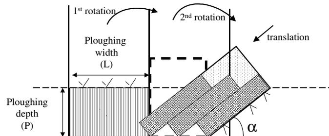
vertical and horizontal co-ordinates of any pixel as a function of its initial co-ordinates, the plowing depth and the plowing width.
